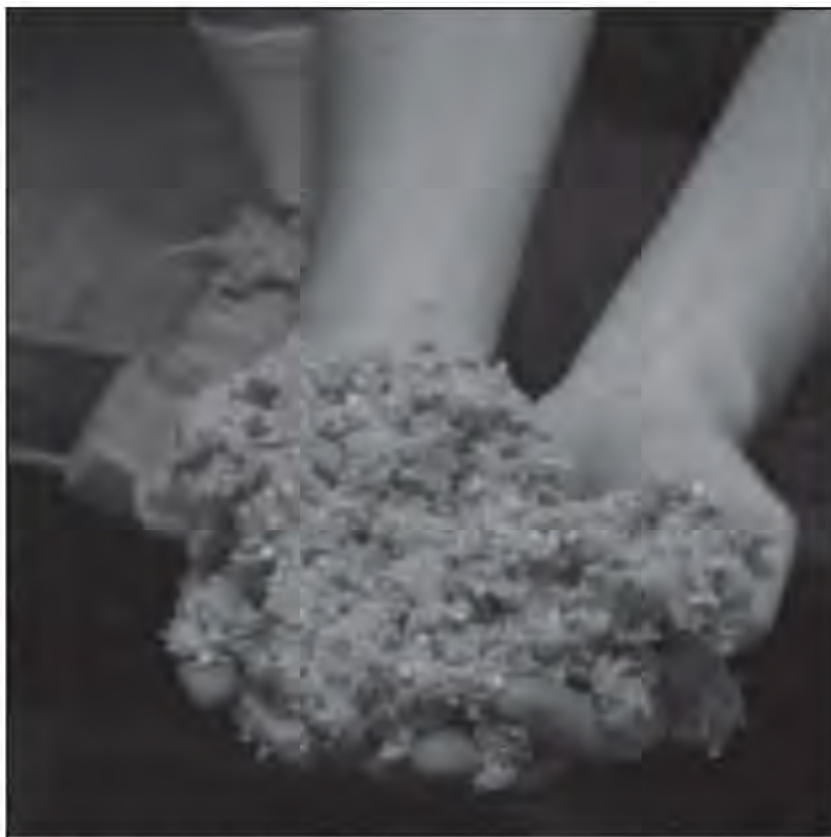
(left) Two handfuls of cellulose insulation. (right) Blowing "loose-fill" insulation
